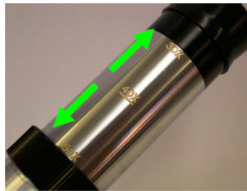
Magnification (30x~50x) Changing with Barrel Up-Down
